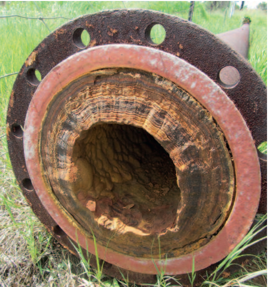
Layers of orange AMD residue have frequently accumulated inside steel pipes. These radioactive materials should be, but have not always been, deposited in a licensed storage facility. © 2012 Bonnie Docherty/IHRC.
