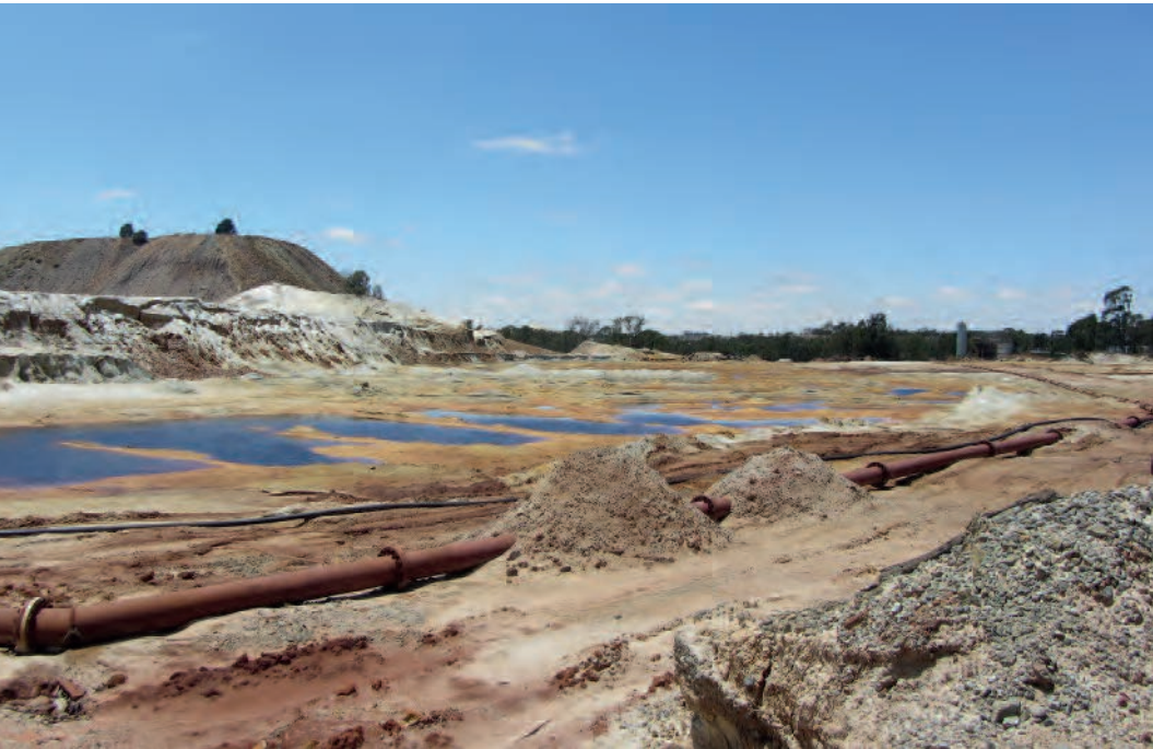
This remining operation, shown in 2014, had almost completely eliminated Sand Dump No. 20 by 2016. While such reclamation has helped address the tailings problem, it must be done carefully because the process stirs up contaminated dust. © 2014 Bonnie Docherty/IHRC.
