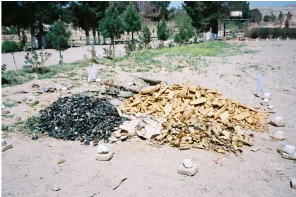
Deminers created these piles of debris as they cleared hundreds of submunitions from a site near Herat, Afghanistan. The black objects are BLU-97 caps, or "spiders." Also visible (clockwise from upper left) are: pieces of cluster munition casings, the yellow foam that surrounds the submunitions, empty submunition canisters, and parachutes. © 2002 Bonnie Docherty/Human Rights Watch
