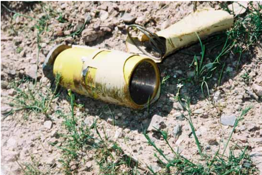
Two BLU-97 submunitions lie in a field near Herat, Afghanistan. The left one is unexploded. Its shaped charge, an anti-armor concave cone, is visible at its right end, and the exterior canister has slipped to expose its antipersonnel fragmentary core. © 2002 Bonnie Docherty/Human Rights Watch
